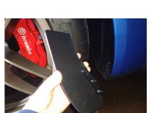
2. The Stone Chip Guards are positioned with the molded offset spacers facing rearward on the car. These spacers allow the Stone Chip Guard to install flush with the wheel well.
